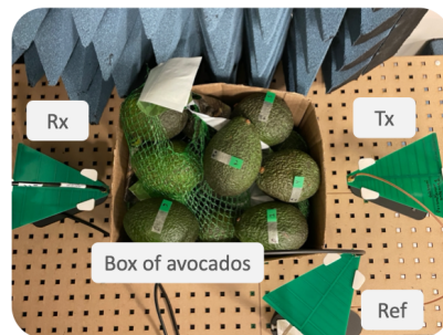
Figure 4: Non-invasive food quality sensing using RF dispersion through densely-packed produce.
