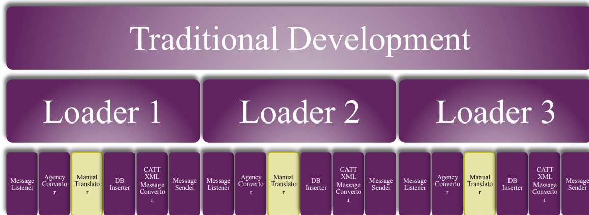
Figure 6: Traditional Development Process. Every loader is developed independently of one another.
