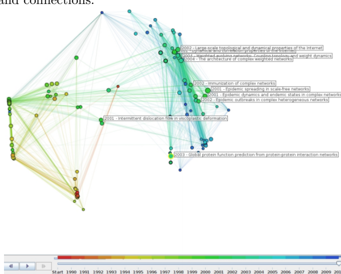
Figure 1: The visualization technique proposed by [3] displays a large node-link diagram that updates at each new time step and uses color to indicate the age of nodes and connections.
