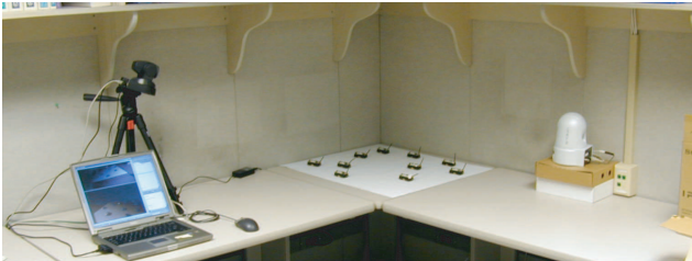
Figure 3. Experimental platform: MicaZ sensor network, laptop, 2 PTZ cameras.
