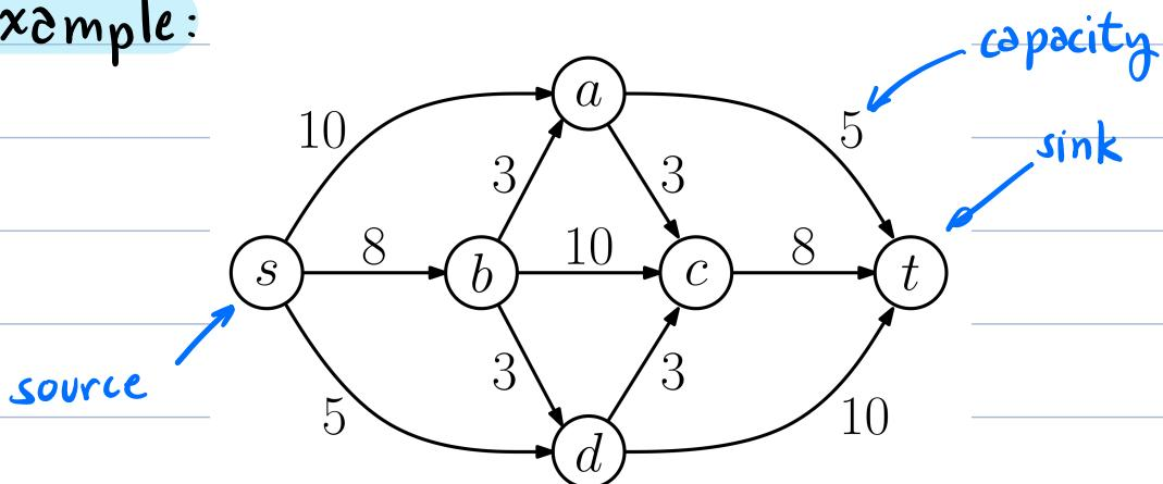
Max-Flow: Thinking of edge  $(u, v)$  as a pipe that can carry  $c(u, v)$  units of flow, how much flow can we push from  $s$  to  $t$ ?
