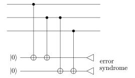
The *error syndrome*, which we get by measuring the ancillas in this circuit, tells us information about the error. In this case, we have the following correspondence between error syndromes and errors:
