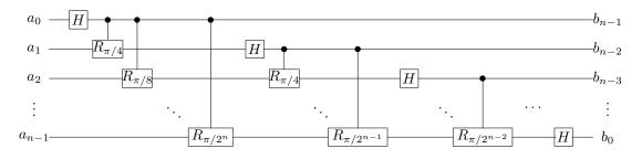
The total complexity of this Fourier transform circuit is  $n + (n-1) + (n-2) + \ldots + 1 = O(n^2)$
