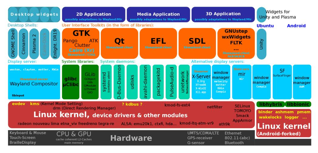
Visible software components of the Linux desktop stack include the <u>display server</u>, <u>widget engines</u>, and some of the more widespread <u>widget toolkits</u>. There are also components not directly visible to end-users, including <u>D-Bus</u> and <u>PulseAudio</u>.
