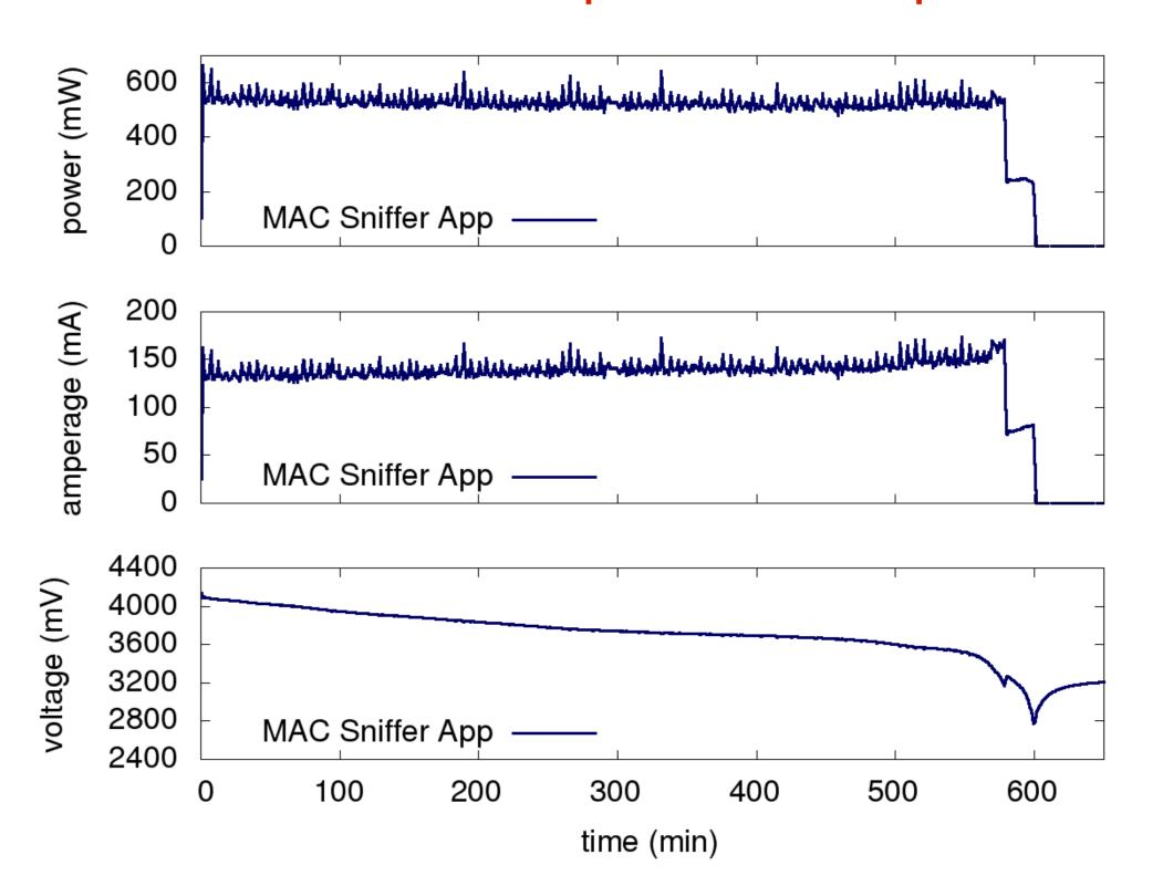
Naively scanning for wifi and bluetooth MAC addresses every 30 seconds drains the phone's battery in about 10 hours, compared to specifications of 6.4 hours of talk time and 11.3 days of standby.
