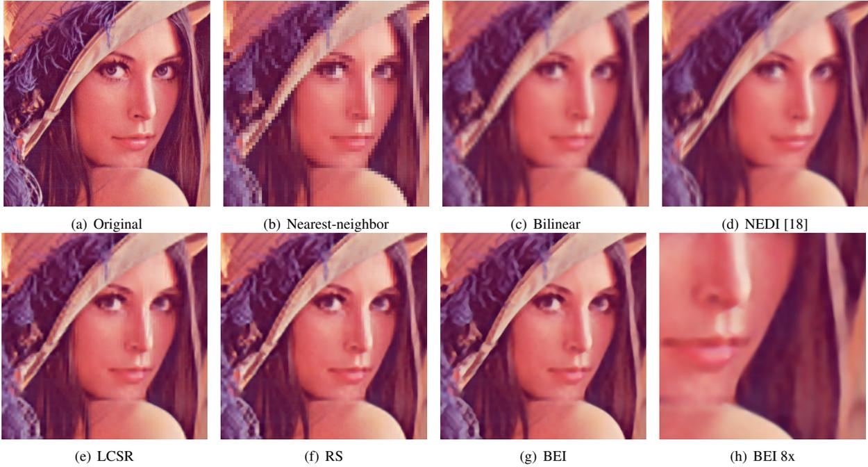
Figure 9. A  $256 \times 256$  region of “Lena” (a) decimated twice and magnified 4x (b – g). Note the gradient steps in (e) and (f), especially in steep gradients such as on the nose and in the shadow on the forehead. Because BEI can model decimation blur explicitly in the capture and recapture processes, it preserves these gradients at 4x (g) and 8x (h) while keeping boundaries sharp.
