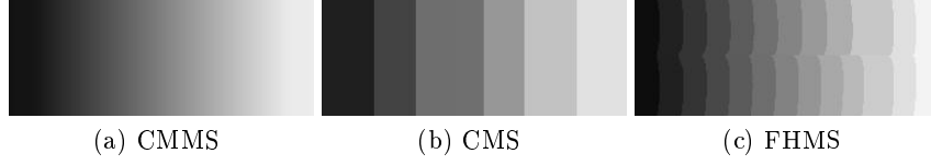
Fig. 1: All the described algorithms applied on a 256 \times 100 pixels smoothly varying image. All the filtering algorithms were executed with spatial resolution h_s = 21 and range resolution h_r = 10 and used a Normal kernel.
