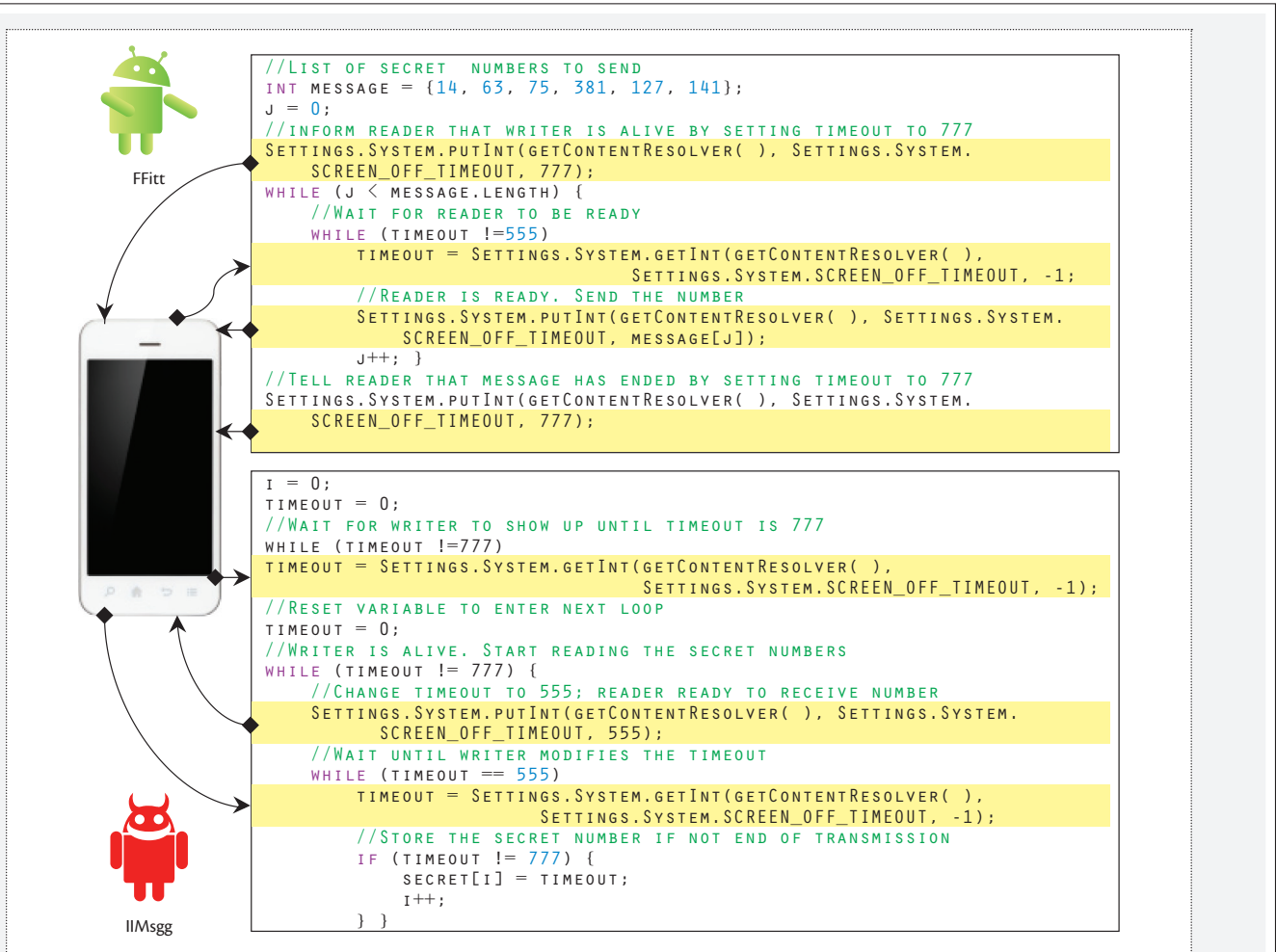
Figure A. A snippet of malicious code embedded in the FFitt and IIMsgg apps that lets them communicate via an unconventional channel: the device’s screen-off time-out. FFitt encodes sensitive fitness and location data as time-out values, which IIMsgg then sends to a contact via a message.
