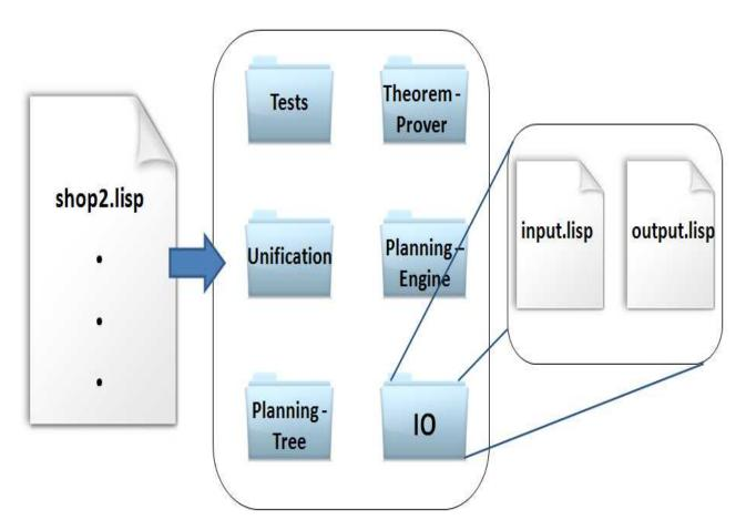
Figure 2: This is an illustration of the reorganization applied to the SHOP2 code. The code began as a single file and was split into subsystems.
