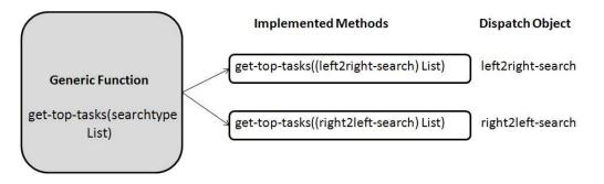
Figure 3: This is an illustration of how method dispatch works in CLOS.
