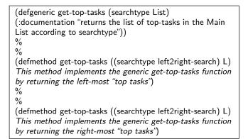
Figure 4: Definition of a generic function and two methods which implement it. Methods are dispatched on the type of the searchtype object.
