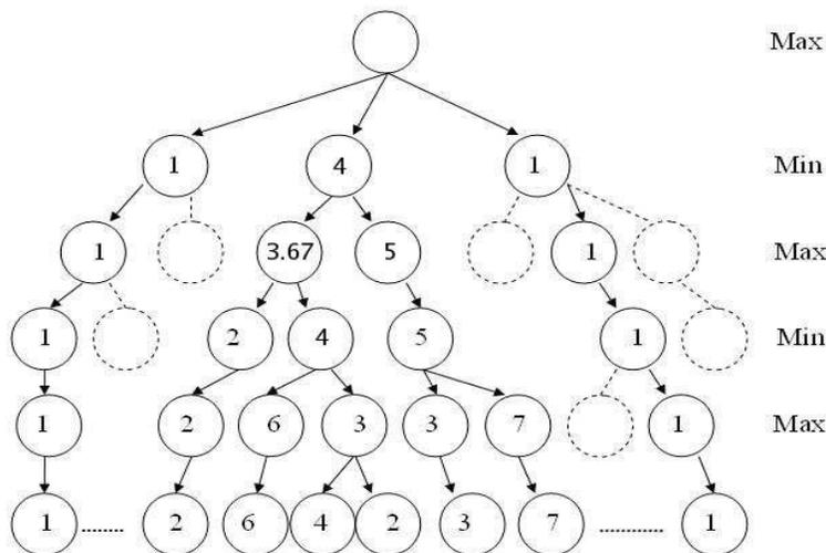
Fig 2. A UCT search highlighting the asymmetric growth of the tree. The value of each node is the arithmetic mean of the value of each child weighted by the frequency of visits.
