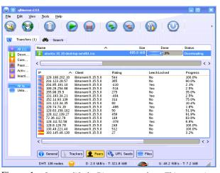
Figure 1: Our modified qBittorrent tracker. This execution includes a LeechLock-enabled peer and shows the divergence between the cooperative peers and the selfish ones. There are 5 properly identified selfish peers in this case.
