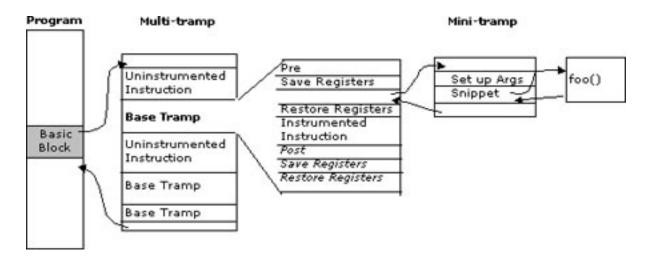
Figure 2: Instrumentation Code Insertion into a Program
