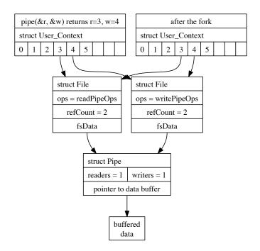
Figure 1: Illustration of the file descriptor table (top), where entries point to struct File objects, after Fork(). There are two struct File objects for the pipe. The pipe object must track whether there are any readers or writers and keep buffered data, the File object must track how many processes (kthreads) hold a reference to the File.
