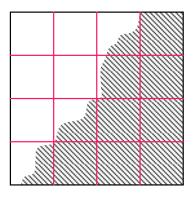
1. initial image decomposition into cells of uniform size
