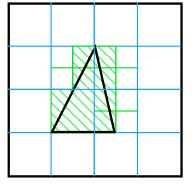
easy to see dependence on perimeter as decomposition only takes place on the boundary as the resolution increases
